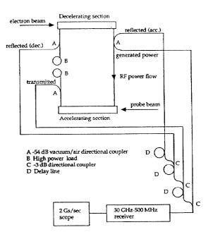
Fig. 4: RF measurements on the CLIC structures
