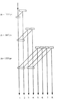
Fig. 2: The eight laser pulse train generator
