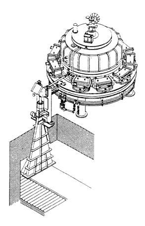
Figure 1: Overall view of the Rhodotron TT200, its beam transport system and scanning horn.
