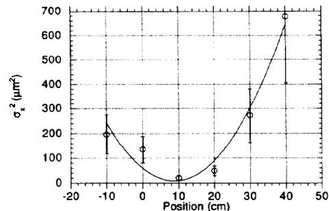
Figure 9. Correlation between the distance to the waist and the measured dimension.
