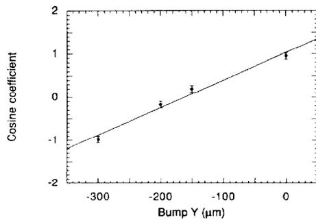
Figure 7. Cosine Fourier coefficient of order 1 of the azimuthal distribution versus the amplitude of a linac bump creating a tail.
