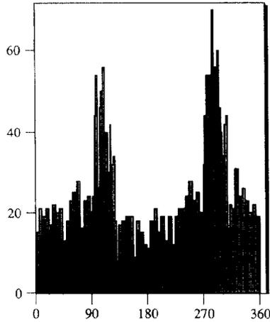
Figure 2. Azimuthal distribution of  $\text{He}^+$  ions (beam size  $\approx 1.3 \times 65 \mu\text{m}$ ).
