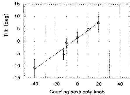
Figure 8. Correlation between a coupling sextupole knob and the measured tilt of the beam.
