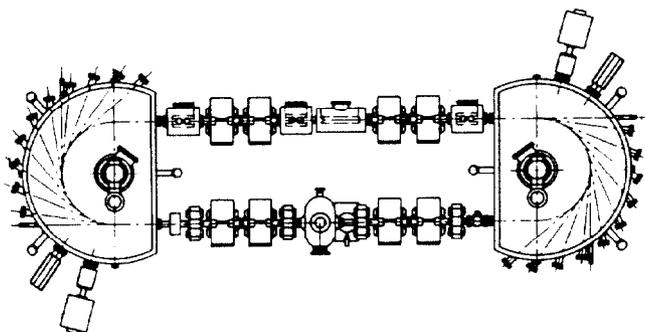
Figure 1. Compact Electron Storage Ring JESCOS, total length 6.5 m
