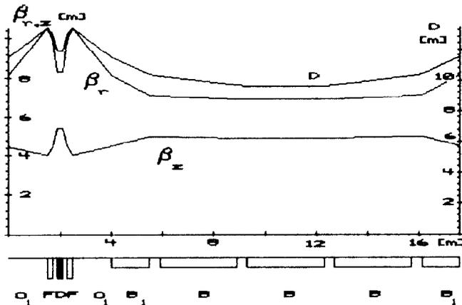
Figure 1. Transverse motion function for one superperiod.
