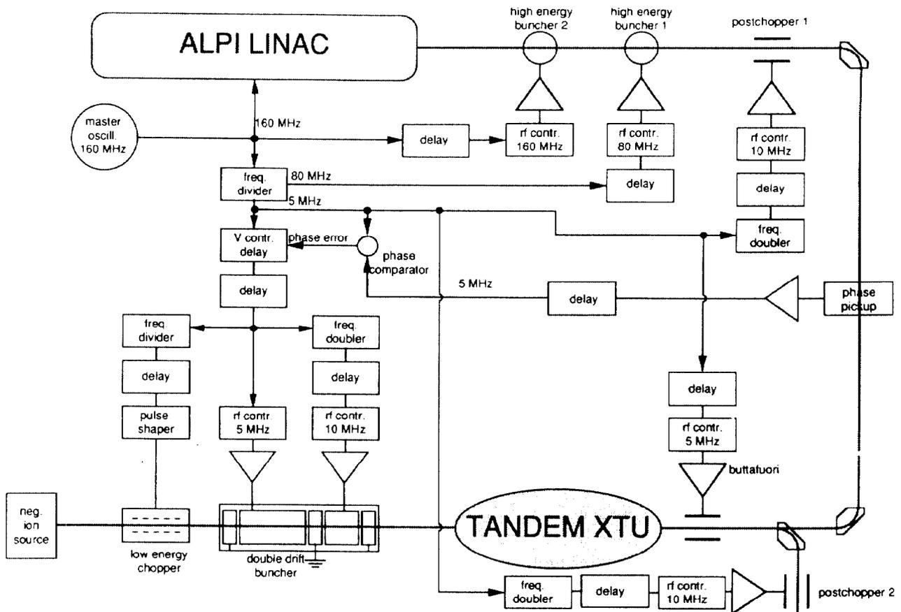
Figure 1: Pulsing system block diagram.
