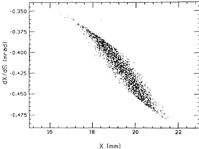
Figure 4: Extracted beam phase space at A0.
