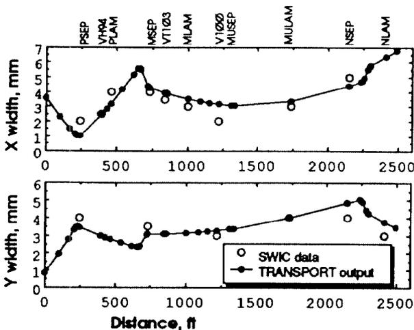
Figure 1: Comparison of SWIC data to TRANSPORT output for the NEUTRINO area.
