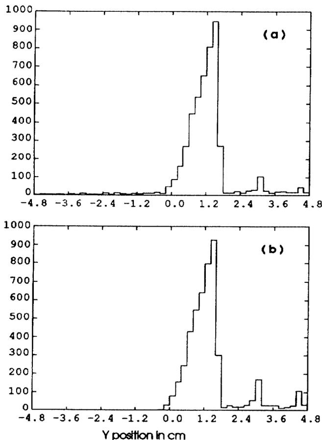
Figure 7: Simulation of Y profile of beam to MESON area at ME2WC, (a) with Coulomb scattering from the PSEP septa wires; (b) without Coulomb scattering.
