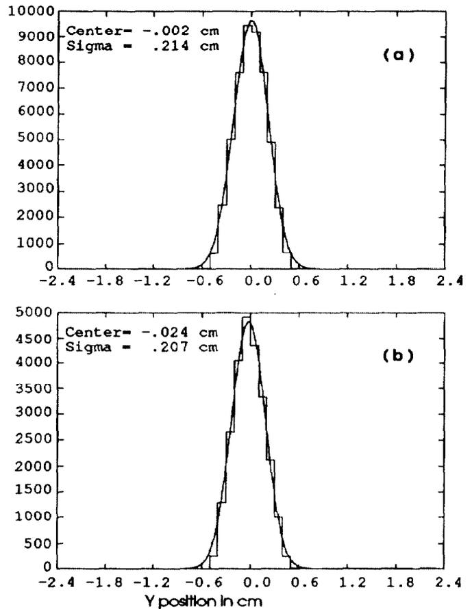
Figure 6: Simulated Y profile of the beam to MESON area at Q203, (a) Single beam; (b) a 50/50 split at PSEP
