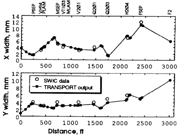
Figure 2: Comparison of SWIC data to TRANSPORT output for the MESON area.
