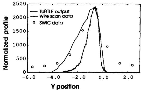
Figure 5: SWIC data, wire scan data, and TURTLE result for split beam profile downstream of PSEP
