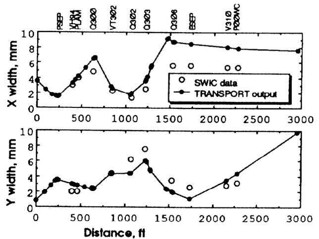
Figure 3: Comparison of SWIC data to TRANSPORT output for the PROTON area.
