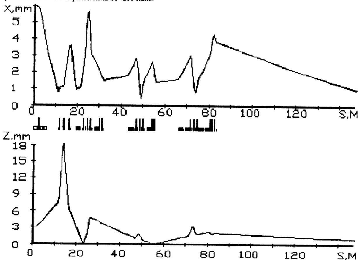
Fig.4 The beam envelopes in PSR-SP channel
