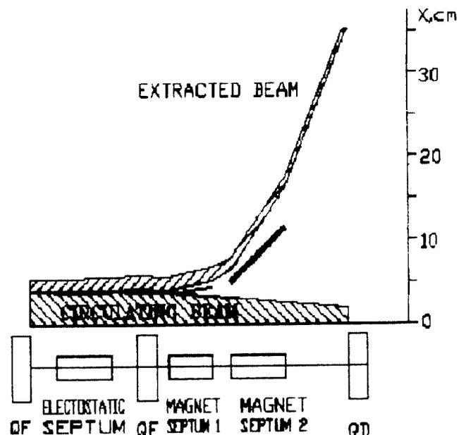
Fig.3 The layout of the equipment for the extraction section
