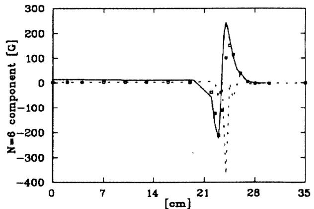
Fig. 3. Variation of dodecapole component with longitudinal position, referred to a radius of 25 mm;  $z=0$  is the magnet centre. Solid line - measured, dashed line - calculated with no end-cut, points - calculated with end-cut.
