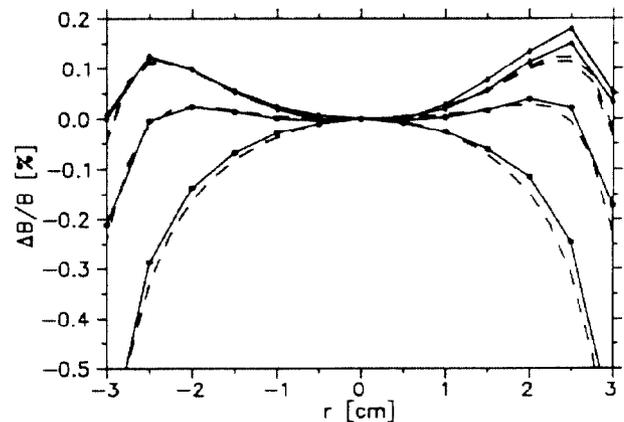
Fig.1 Field homogeneity in the centre of the dipole magnet at various current levels : 200 A (upper curves), 600 A, 800 A and 1000 A (lowest curves); solid lines - measurements, dashed lines - calculations.
