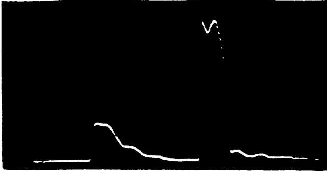
Figure 6: Result of measurement, input pulse 5  $\mu\text{sec}$ , output  $\approx 1 \mu\text{sec}$ , gain 5.4...5.6 dB
