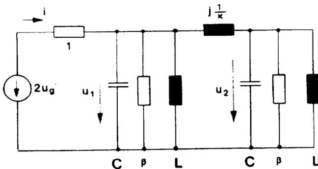
Figure 1: Equivalent circuit for two coupled cavities
