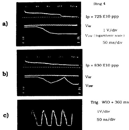
Fig. 13 Stability Improvement by Bucket Deformation.
