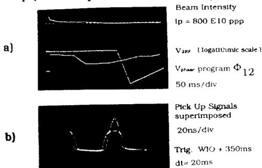
Fig. 11 Bunch Shape Control.
