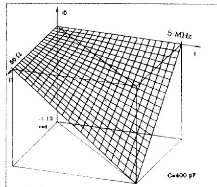
Fig. 3. Phase Angle  $\phi$  vs frequency  $f$  and resistance  $R$ .
