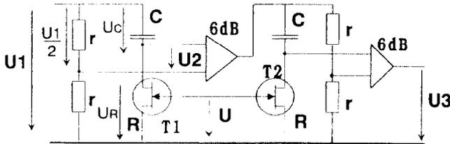
Fig. 1 Schematic Diagram of Phase Shifter.
