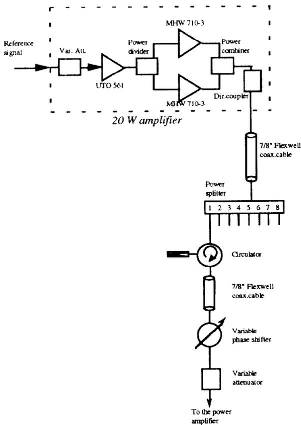
Fig. 1 Block diagram of the RF distribution system
