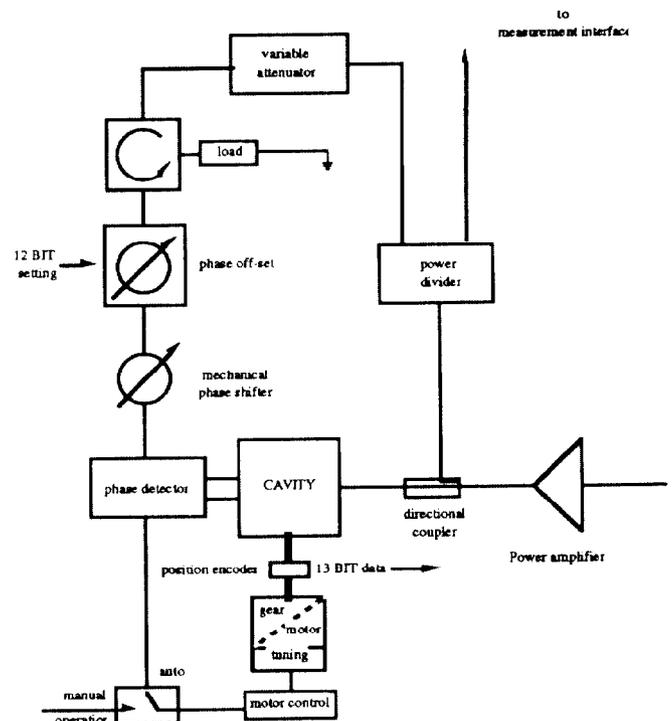
Fig.2 Block diagram of the mechanical tuning loop.
