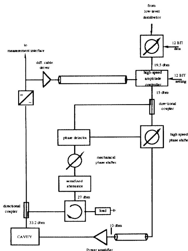
Fig. 3 Block diagram of the fast phase and amplitude feedback loops
