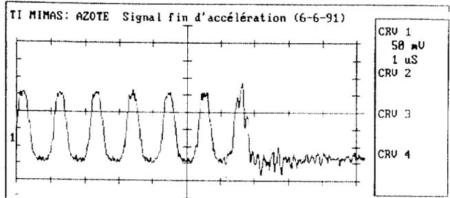
**Figure 5** : The last acceleration turns of a  $N^{7+}$  beam (peak intensity : 400  $\mu A$ ).
