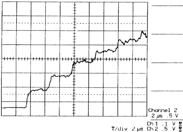
**Figure 4** : Intensity increase during the injection of a high intensity beam (increase = 1 mA/turn).
