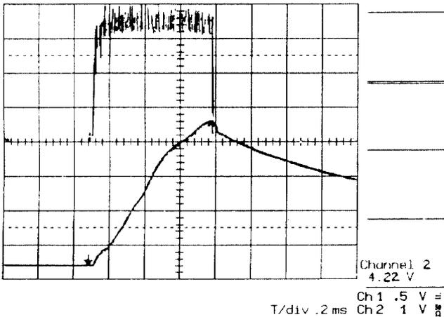
**Figure 3** Injection of a high intensity (80 mA peak) light ion beam.
