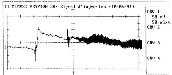
**Figure 6** : Injection of a krypton  $30^+$  beam (peak intensity : 600 nA).
