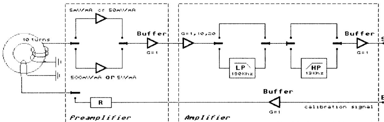
Figure 2 - Beam transformer electronics
