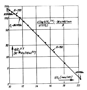
Fig. 3: Fowler-Nordheim plot of integrated dark current Q versus electric field  $E_C$  on copper cathode
