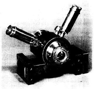
Fig. 1: RF-Gun and Waveguide viewed from beam exit. Each cell has a piston tuner and a field monitor.
