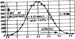
Fig. 4: Beam momentum p versus number dN of particles measured after bending magnet BHZ 190, Number of particles at gun exit:  $1.7 \times 10^{11}$
