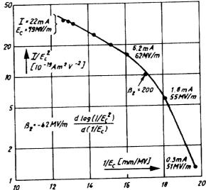
Fig. 5: Dark current I versus electric field E<sub>C</sub> on CsI-photocathode, plotted for field induced hot electron emission<sup>5</sup>)
