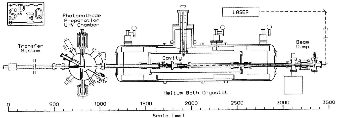
Figure 2: Complete Experimental Setup
