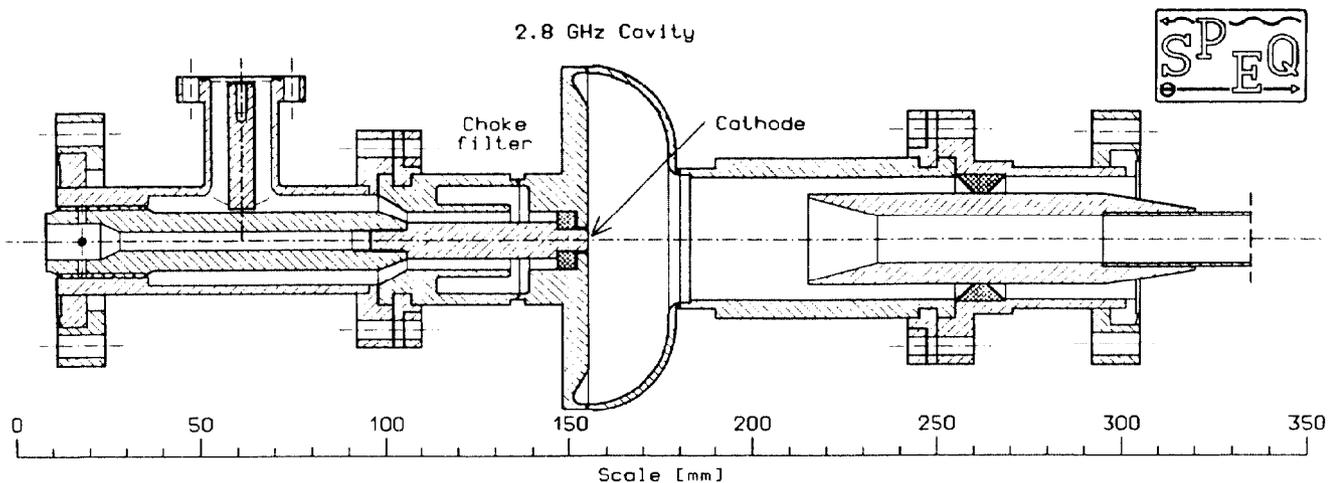
Figure 1: 2.834 GHz Superconducting Cavity Setup
