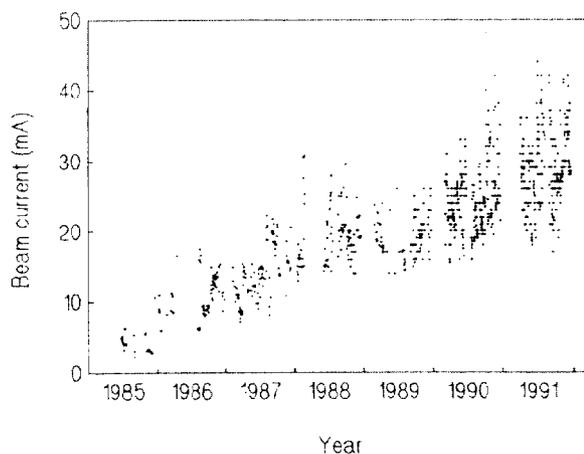
Fig 5. Recorded H<sup>-</sup> current from operational sources.
