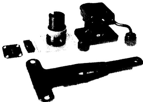
Fig 1. Ion source components. l to r: extraction slit plate; anode; cathode; ion source body; & below: extraction electrode.
