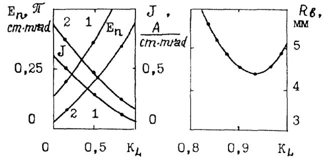
Fig. 6. Dependences of  $E_n$ ,  $J$  and minimal proton beam radius  $R_b$  on value  $K_1$ : 1-90% of particles; 2-50%;  $K_1=0,57$ ; for EP1, EX2, SL1.
