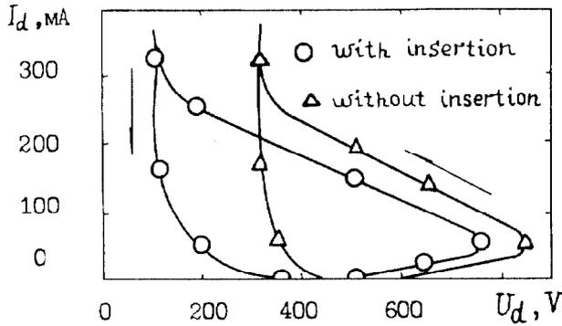
Fig.2. Dependence of discharge voltage  $U_d$  on discharge current  $I_d$  for modified cathode system.
