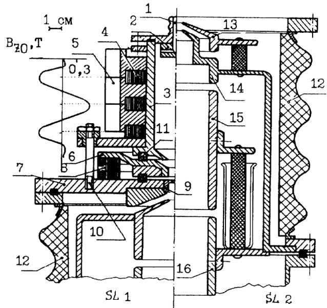
Fig.1. The geometry of plasma generator and of ion optical system (the details see in text).
