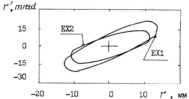
Fig.3. Emittance diagrams of proton beam for EX1 and EX2 extraction systems.
