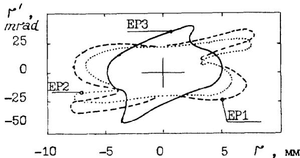
Fig. 5. Emittance diagrams of proton beam:  $I_d=10$  A; gas pressure 5 Pa;  $K_1=0,57$ ;  $K_2=0,964$ ; beam energy 80 keV.
