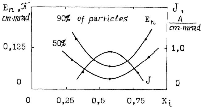
Fig. 4. Dependences of normalized emittance  $E_n$  and phase density  $J$  of proton beam on coefficient value  $K_1$  with EX2 and EP1
