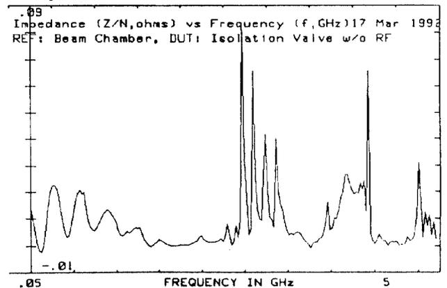
Fig. 2 Broadband impedance for the valve w/o RF shielding
