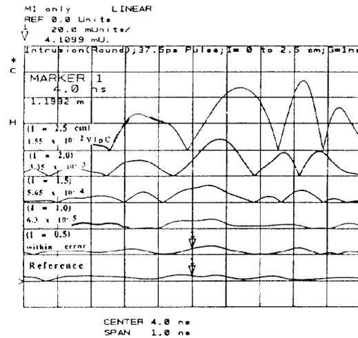
Fig. 4 TD transform of the S11 for the round intrusion with I = 0 to 2.5 cm and their loss factor, k.
