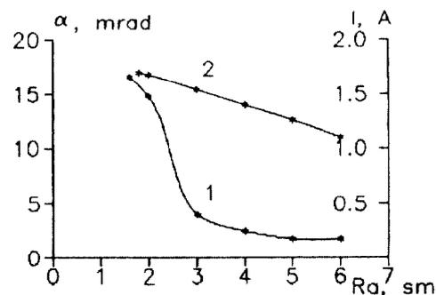
Fig 2. The velocity angle spread (1) and electron beam current (2) vs the anode hole radius
