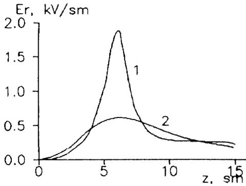
Fig 3. Axial distribution of the electric field on the electron beam edge. The radii of the anode hole of 2 and 4 sm correspond to curves 1,2.
