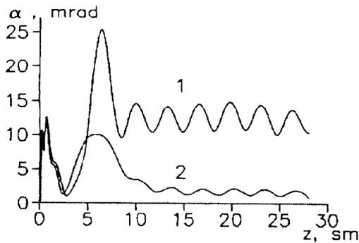
Fig 4. The variation of the electron beamangle spread along the system. The radii of the anode hole of 2 and 4 sm correspond to curves 1,2.
