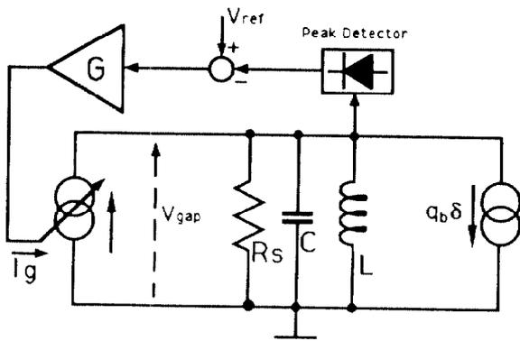
Figure 5. Equivalent Circuit for the Tracking Code
