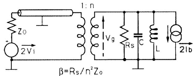
Figure 1. Circuitual Model of DAΦNE RF System
