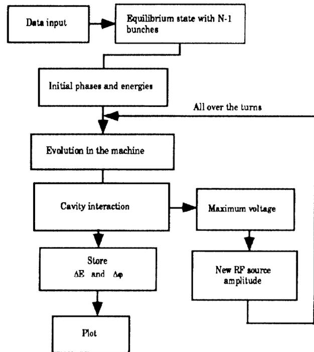
Figure 4. Tracking Code Flow Chart
