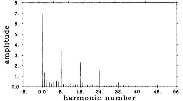
Figure 2: Spectrum of the parasitic skew gradient
