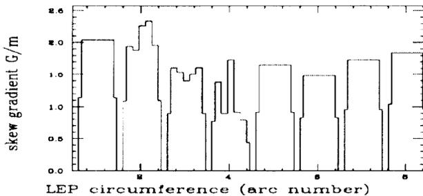
Figure 1: Azimuthal distribution of the skew gradient
