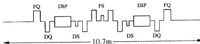
Figure 1. Unit Cell of the Circular Machine
