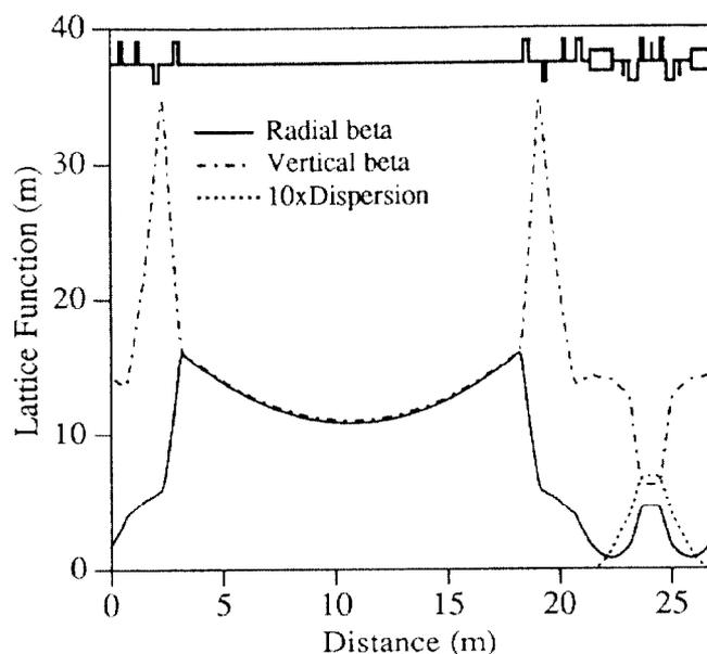
Figure 5. Lattice Functions of the DAPS Long Cell
