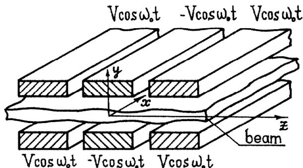
Fig. 1. Schematic representation of RF accelerating channel with a ribbon beam.
