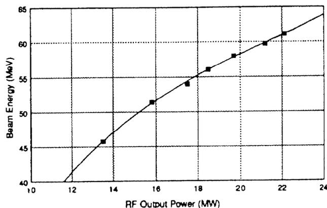
Figure 3: Achieved beam energy and klystron output power
