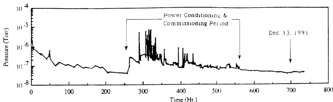
Figure 2: Vacuum pressure history of the preinjector linac
