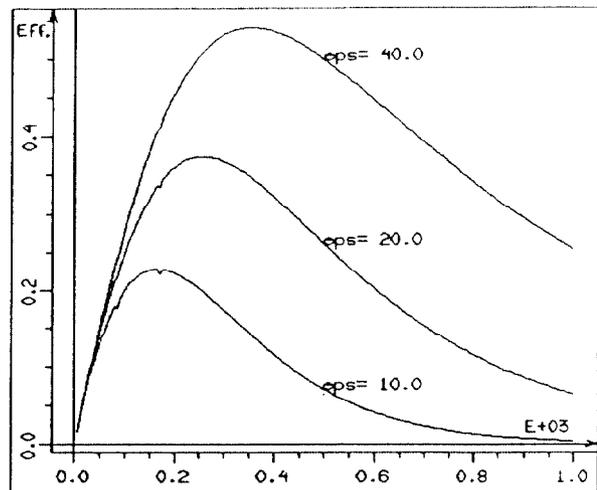
Figure 3 Computed efficiencies of semi-slow extraction versus the acceleration speed (Hz/ms) to the resonance for different beam emittances (95%) and for  $(\frac{\Delta p}{p})_{4\sigma} = 1\text{‰}$ .
