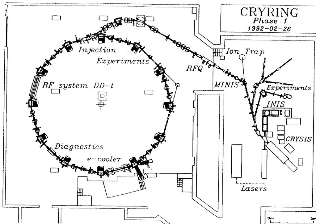
Figure 2: Layout of the CRYRING project, phase 1.
