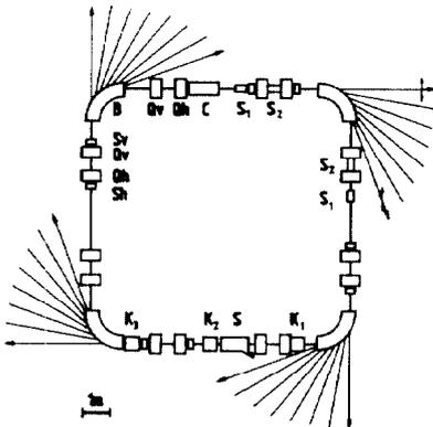
Fig. 1: Schematic layout of a general-purpose compact synchrotron radiation source as studied at Karlsruhe.
