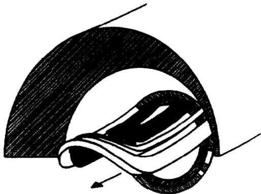
Fig. 3: 3D view of the end of the bending magnet.
