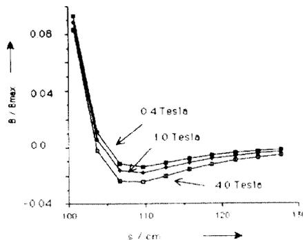
Fig. 5: Field along the reference orbit in the end region. The inner radius of the iron is 14 cm. s = 0 corresponds to the center of the magnet.
