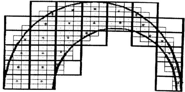
Fig. 2: Discretization of the torus for the first iteration step.
