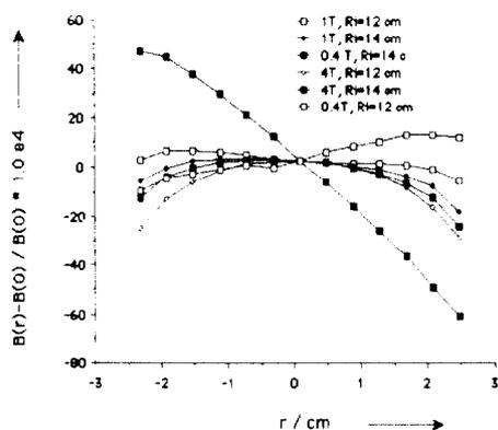
Fig. 4: Relative field deviation in the center of the magnet for the two inner radii of iron of 12 and 14 cm.
