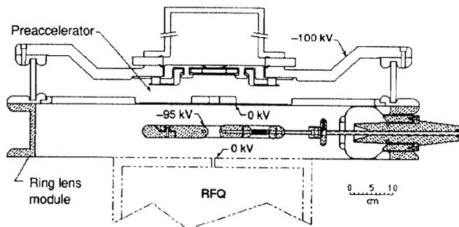
Fig. 1b. Preaccelerator with ring lens only.
