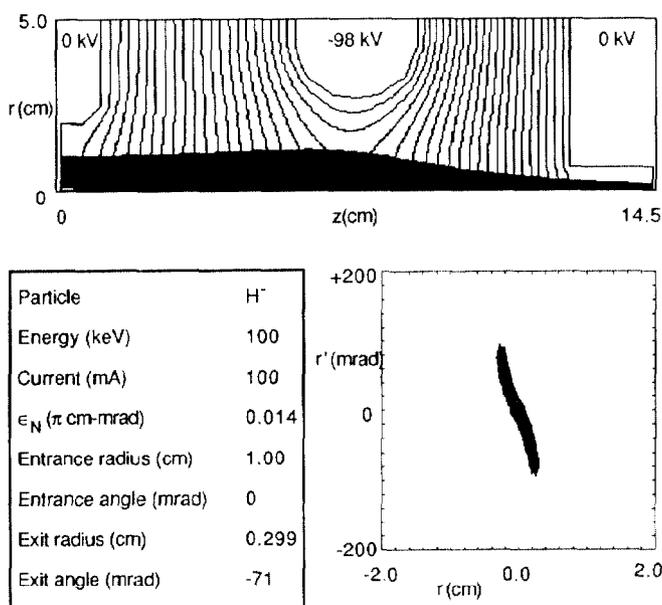
Fig. 3. Sample particle simulation of the axisymmetric lens for RFQ matching, showing the beamlet trajectories and the phase plot at 12.6 cm, the location of the simulated RFQ entrance. The beam radius is 3 mm at this point and decreases toward the RFQ match point.
