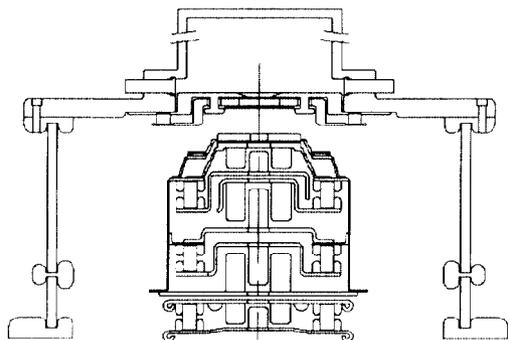
Fig. 1a. Preaccelerator and quadruplet ESQ LEBT; ring lens not shown.
