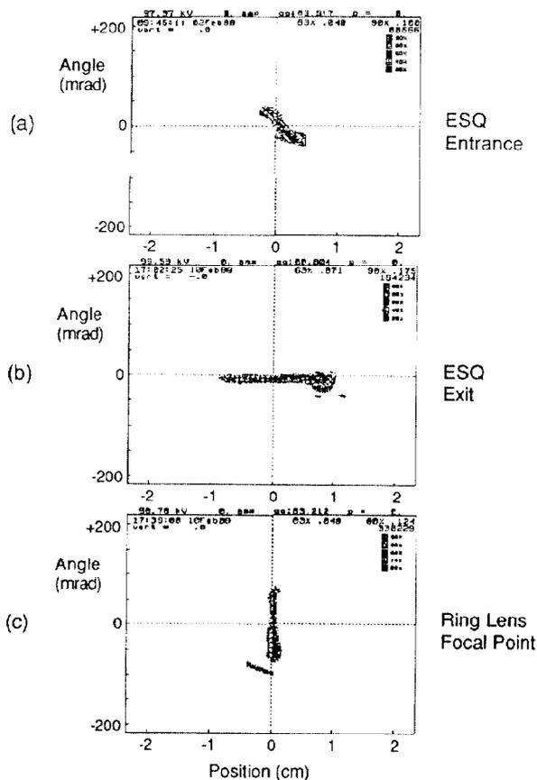
Fig. 5. Emittance scans projected back to: (a) the ESQ entrance; (b) the ESQ exit; and (c) the ring lens focal point. The larger phase space area seen in (b) is probably an instrumental effect. In (a) and (c) the normalized emittance is about  $0.025 \pi$  mrad-cm.
