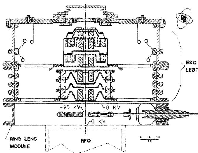
Fig. 4. Prototype LEBT shown with ring lens, as tested. The ring is supported by three feed through insulators, one of which is seen here (see text). The hypothetical RFQ entrance region shown schematically with dotted lines is replaced experimentally by the exit electrode described in the text.
