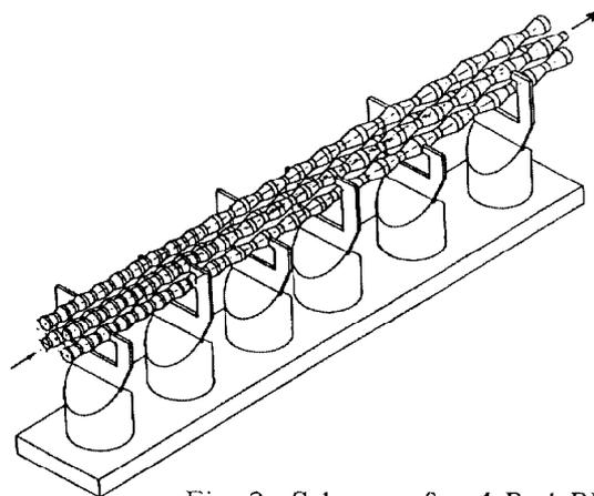
Fig. 2 Scheme of a 4-Rod RFQ
