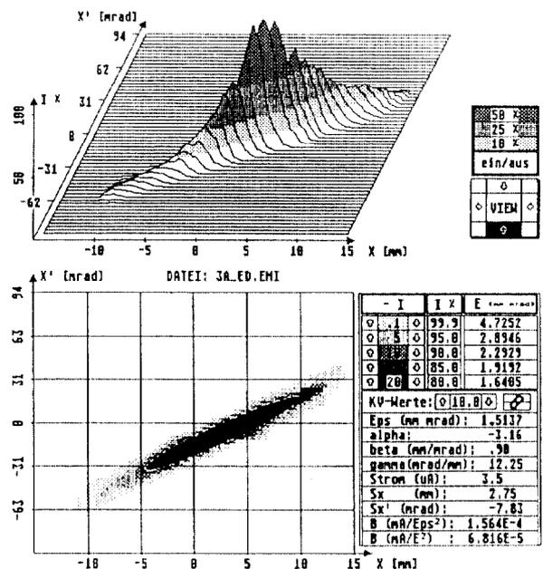
Fig. 5 Measured radial beam emittance
