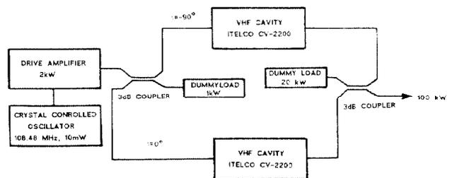
Fig. 8 Block diagram of the rf-transmitter
