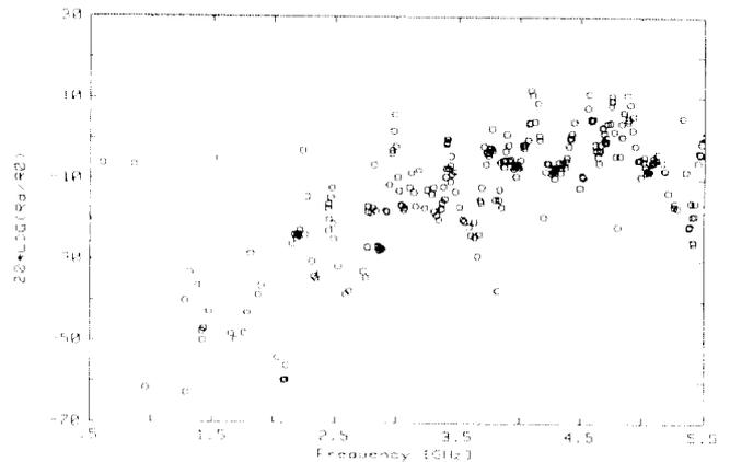
Fig.3: Spectrum of (a) the undamped and (b) the damped test cavity.
