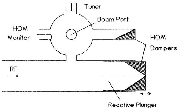
Fig 1: Sketch of cavity with RF feed and HOM damper.
