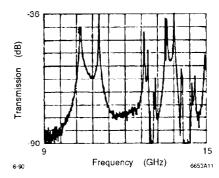
Figure 10: Track 4 single cavity resonances with waveguides shorted.
