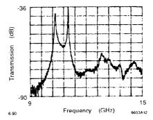
Figure 11: Track 4 single cavity resonances with waveguides terminated.
