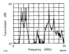
Figure 8: Track 3 with A-B probe coupling and waveguides terminated.
