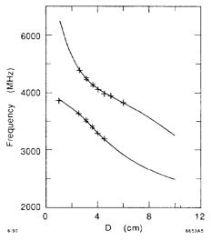
Figure 4: Measured single-cavity Track 2 waveguide resonance frequencies as a function of waveguide length, compared to the predictions of ref. 3.
