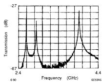
Figure 5: Single-cavity Track 2 resonances coupled to terminated waveguides.
