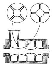
Figure 1: Cross-sections of Track 1 slotted disk structure.
