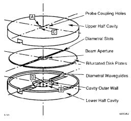
Figure 2: Single-cavity Track 2 with half-disks.
