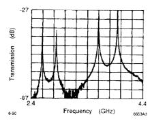
Figure 3: Single-cavity Track 2 resonances decoupled from waveguides.
