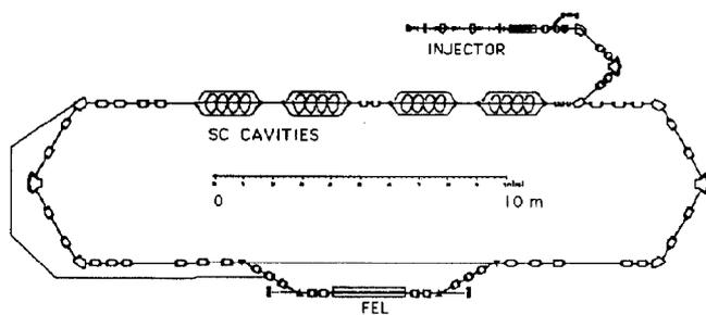
Fig. 1 - Schematic Layout of LISA Accelerator.
