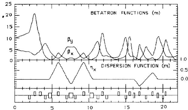
Fig. 4 - Optical Functions from SC Linac to FEL.
