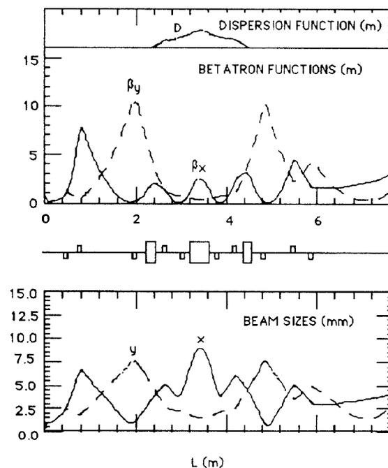
Fig. 3 - Optical Functions Along 1 MeV Bend.
