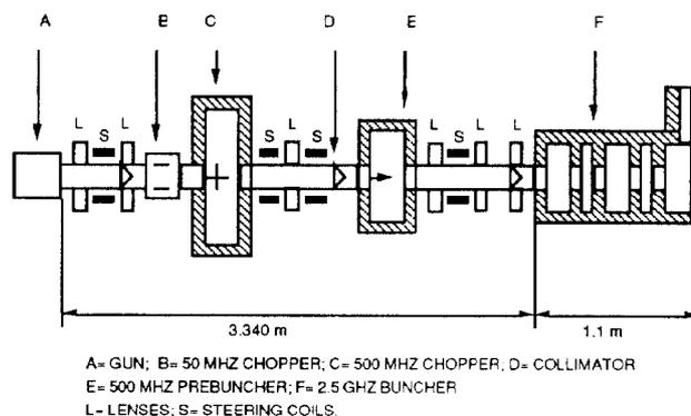
Fig. 2 - Sketch of the Injector.
