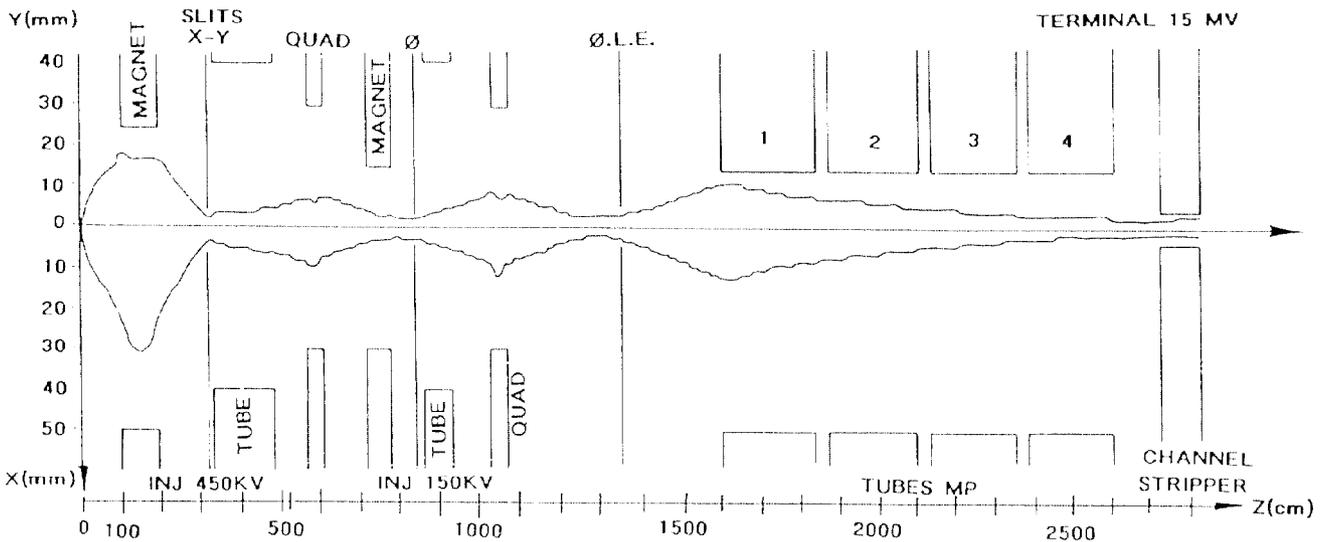
Fig.3 Tandem beam optic.
