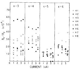
Fig. 7 Integrated harmonic contents measured for the eight superconducting quadrupole magnets fabricated.
