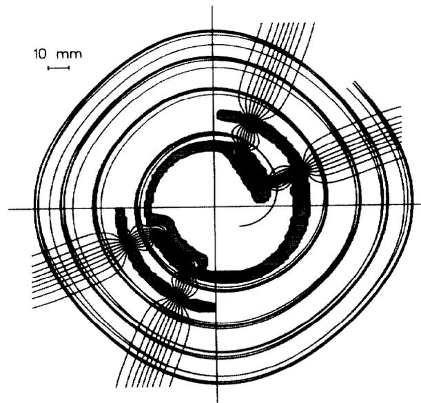
Fig. 3. Orbits of rays with 5 different starting times. Also shown are the central region electrodes in the median plane and the equipotentials of the electric field.
