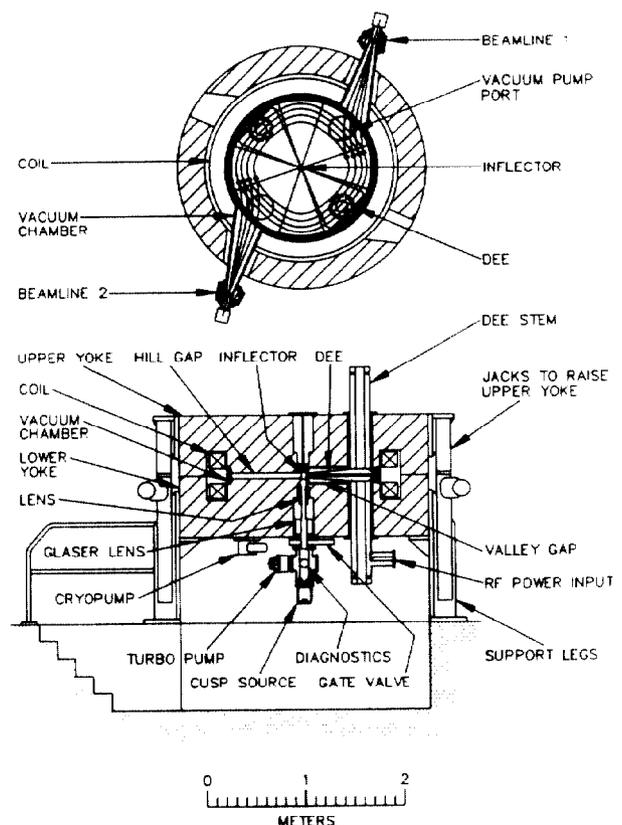
Fig. 1. Cross-sectional and plan views of the cyclotron.
