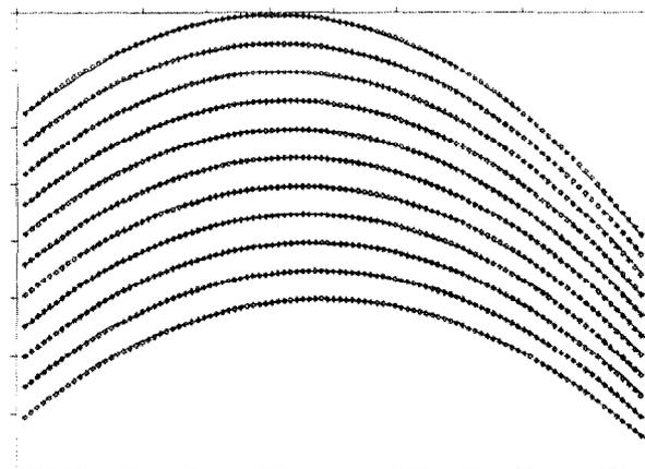
Figure 7: Rays for the determination of  $c_x$  and  $c'_x$ . Here  $-5mm \leq x_0 \leq 5mm$  and  $x'_0 = y_0 = y'_0 = \delta = 0$ , i. e. the rays start out in the median plane parallel to the central ray. The focusing effect is quite noticeable at the end of the system.
