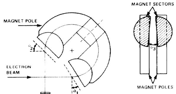
Figure 5: Enge single-magnet achromat: angles  $\alpha_1, \alpha_2,$  and  $\alpha_3$  can be adjusted by moveable shims to satisfy optical constraints. From [8].
