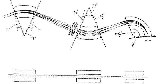
Figure 3: Three-magnet alternate achromat: median plane lay-out. From [6].
