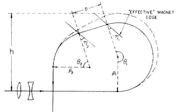
Figure 4: Two-dipole achromat with input quadrupoles. This design minimizes distance  $h$ . From [7].
