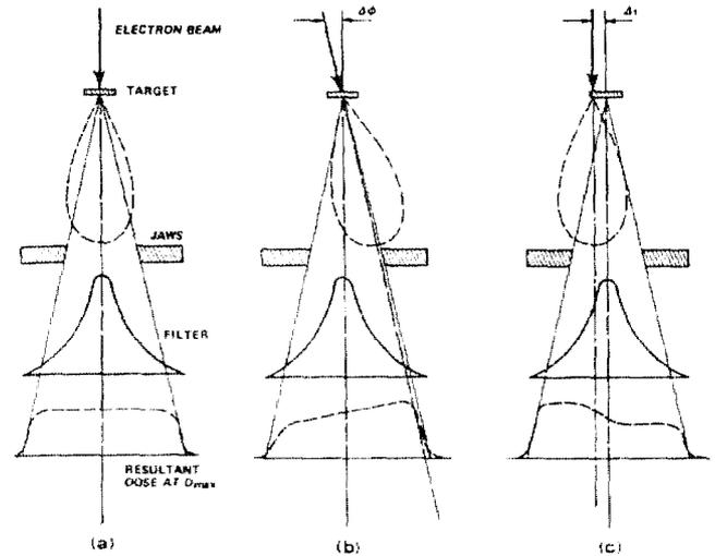
Figure 1: Resultant X-ray dose distribution for: (a) properly aligned beam, (b) beam with an angular divergence  $\Delta\phi$ , (c) beam with a radial displacement  $\Delta r$ . From [1].
