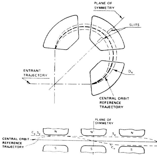
Figure 2: Three-sector achromat: cross-section view in the bend and the cross plane. From [1].
