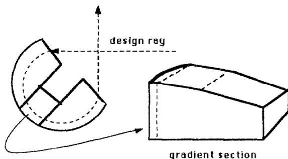
Figure 6: Schematic view of the Siemens magnet. Non-uniform field in the middle section is produced by two poles shaped as shown.
