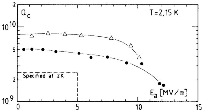
Fig.4: Cavity's  $Q$  as a function of accelerating field of the cavities # 1 ( $\bullet$ ) and 3 ( $\Delta$ ) after the titanium treatment, assembled to a sealed cavity pair
