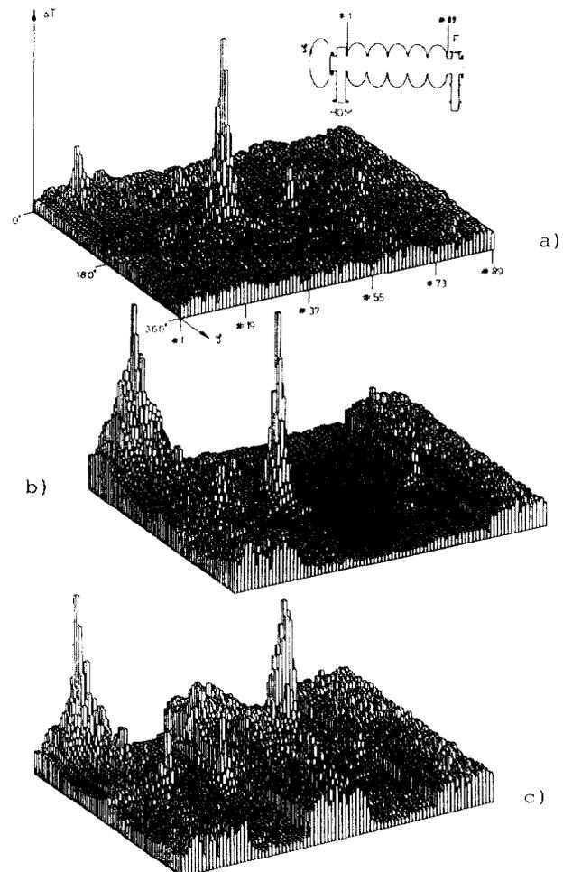
**Fig. 3:** Temperature maps of cavity # 3 taken in the accelerating ( $\pi$ ) (a),  $4/5 \pi$  (b) and  $3/5 \pi$  (c) mode
