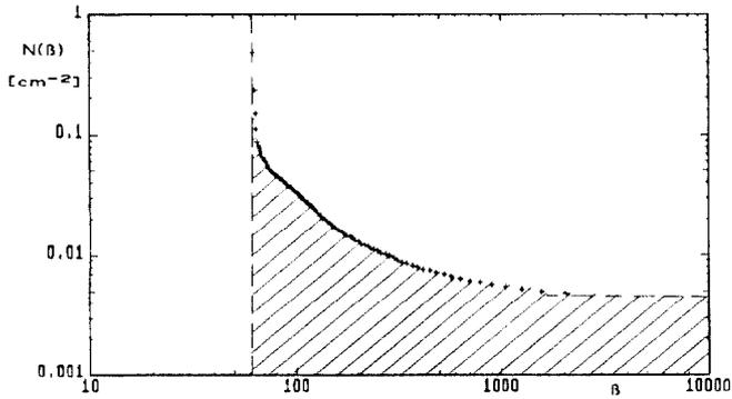
Fig. 6: Upper limit for the density of electron emitters in a 3 GHz single-cell cavity as a function of the anomalous field enhancement factor  $\beta = E_{th} / 63.8$  MV/m. The shaded region represents the best performance achieved in cavity S3.
