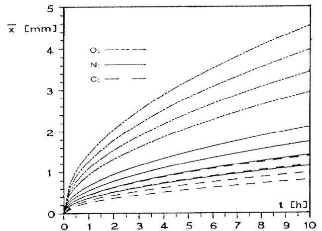
Fig. 1: Diffusion lengths of the main interstitial impurities O, N and C in Nb as a function of annealing time. Each set of four lines correspond to temperatures between 1200°C and 1350°C in 50°C steps, respectively.
