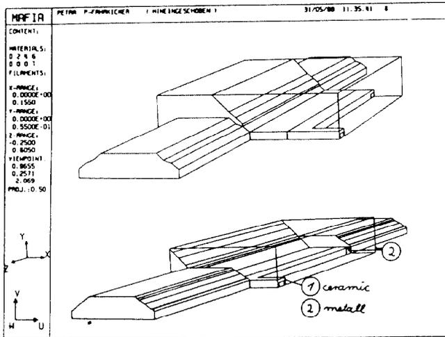
Figure 2: Second design of the removable ejection kicker. The upper picture shows the kicker with the magnet inside the tube. The lower picture shows the magnet totally removed from the tube.
