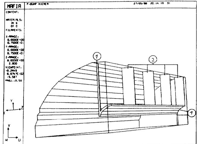
Figure 3: proton beam-dump kicker. One quarter of the structure is shown. Parts marked with 1 are metall, those marked with 2 are dielectric with ε=3.5.
