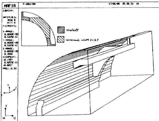
Figure 4: Beam position monitor The figure shows one-eighth of the monitor.
