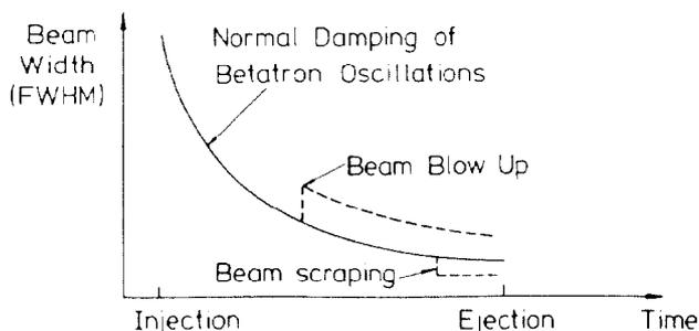
Fig. 5: Illustration of Beam Width During Acceleration (Display is obtainable from either of above types of profiles)
