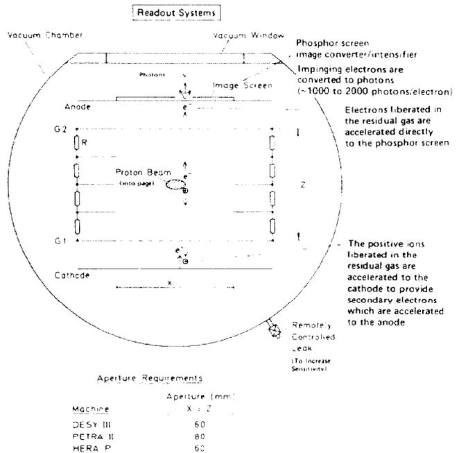
Fig. 1: Cross Sectional Schematic of the Proton Beam Imaging Component of the Residual Gas Ionization Profile Monitor
