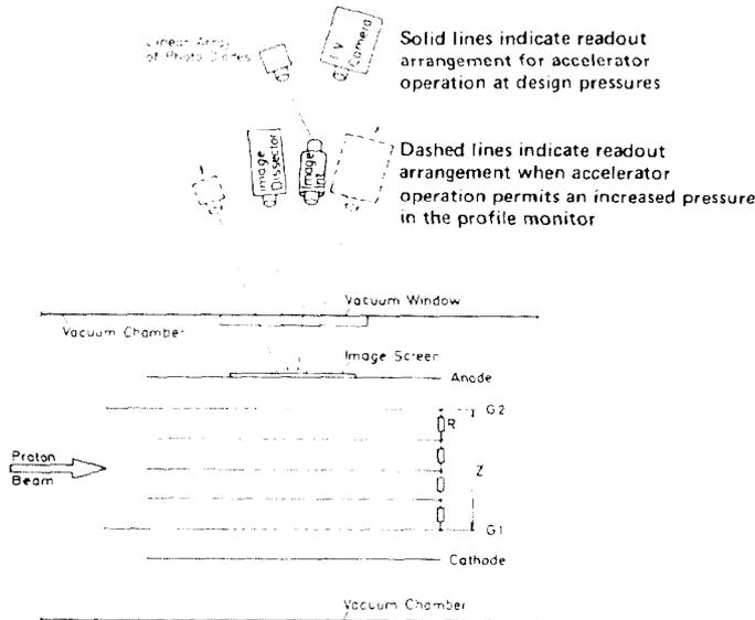
Fig. 2: Schematic of Profile Monitor System with Multiple Readouts
