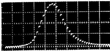
Fig. 3: Expected Profile from Linear Array of Photodiodes
