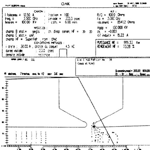
Figure 5 - Bunch motions in an output cavity - Bad Bz
