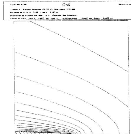
Figure 1 - OAK : Equipotentials in the region around an ellipsoidal needle
