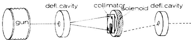
Fig. 3 Scheme of the chopper system
