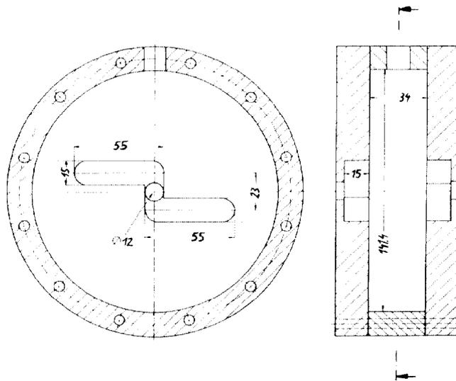
Fig. 5 The chopper cavities.
