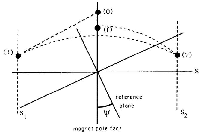
Figure 1: Midplane geometry. Reference plane is normal to the design trajectory.
