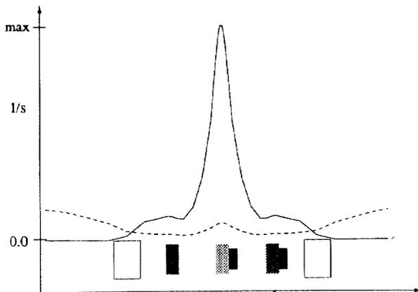
Fig 5. Relative growth rates due to IBS for a cooled beam for two different working points. Dashed line:  $Q_x=2.3$ , solid line:  $Q_x=3.3$ .
