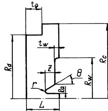
Fig. 1. Geometrical notation of a half-cell DAW cavities.
