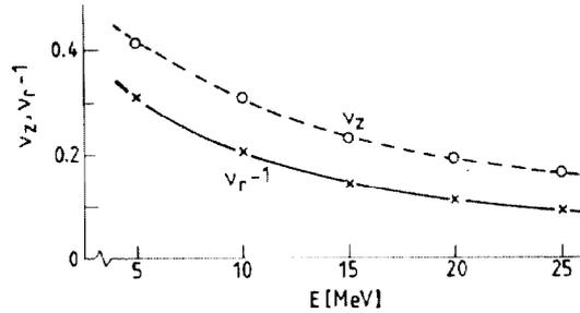
Fig. 3: Horizontal and vertical tunes for equilibrium orbits.
