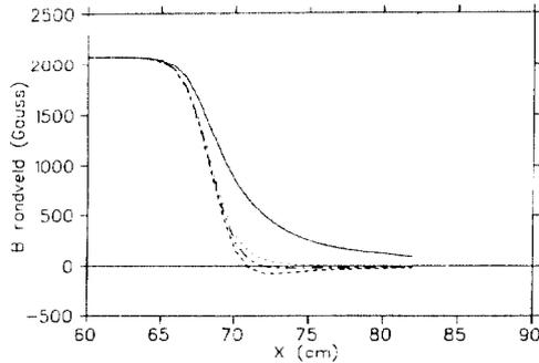
Fig. 2: Effect of field clamps at the entrance of the dipole: solid line: no field clamp, dashed lines: plus, zero, minus excitation of the field clamp.
