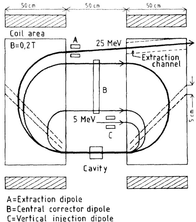
Fig. 1: Microtron lay-out.
