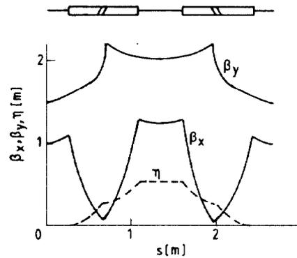
Fig. 4: Dispersion and beta functions at 15 MeV.
