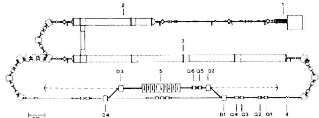
Fig. 2 Part of the accelerator with the planned FEL experiment (1) electrostatic preaccelerator, (2) superconducting injector, (3) superconducting linac, (4) first recirculation, (5) undulator magnet, (Q1-6) quadrupole magnets, (D1-4) dipole magnets
