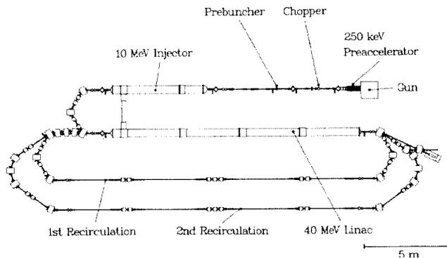
Fig. 1 Layout of the 130 MeV accelerator
