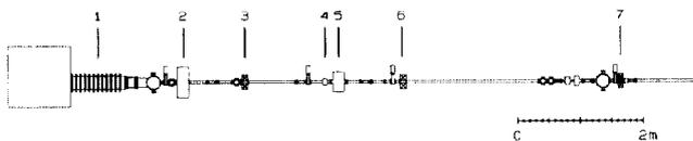
Fig. 3 Layout of the high current 250 keV injector from the electron gun to the begin of the superconducting capture section (1) electrostatic preaccelerator, (2) subharmonic chopper resonator, (3,6,7) solenoid lenses, (4) chopper orifice, (5) subharmonic buncher resonator
