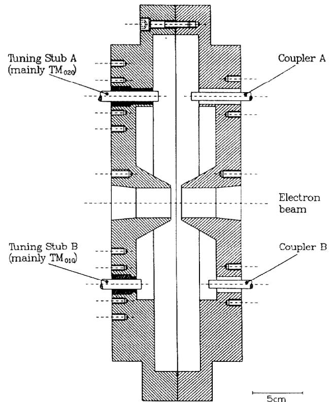
Fig. 4 Mechanical layout of the subharmonic single cavity double frequency buncher resonator
