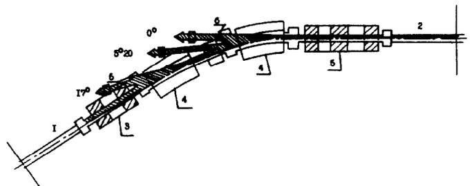
Fig. 5. Plan view of one sector of the storage ring showing radiation transmitted to the beam lines.
