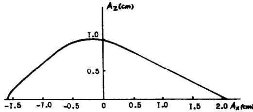
Fig. 3. Dynamic aperture of the magnetic structure of Siberia-2.
