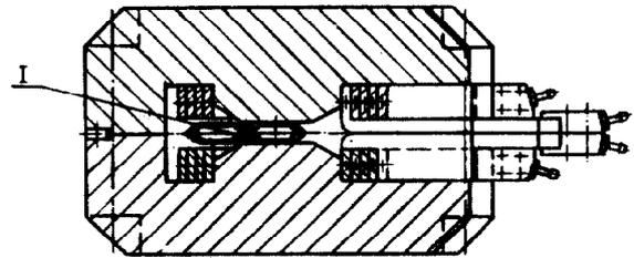
Fig. 4a. Storage ring bending magnet cross section.
