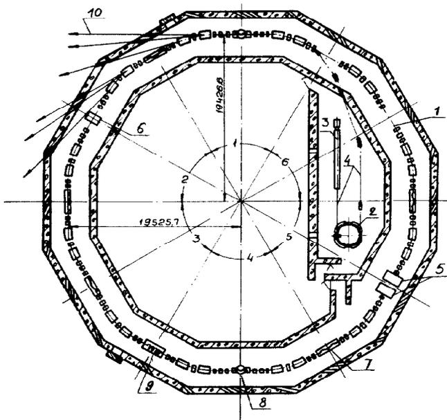
Fig. 1. Schematic of SR source «Siberia-2» showing the injection system (100 MeV linac (3)) a 450 MeV booster storage ring Siberia-1, (2) transport lines, storage ring lattice (1) and SR beam lines (10).
