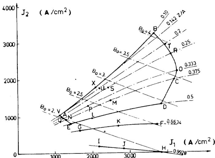
Fig.4 - Cyclotron operating diagram in the (J1, J2) plane.
