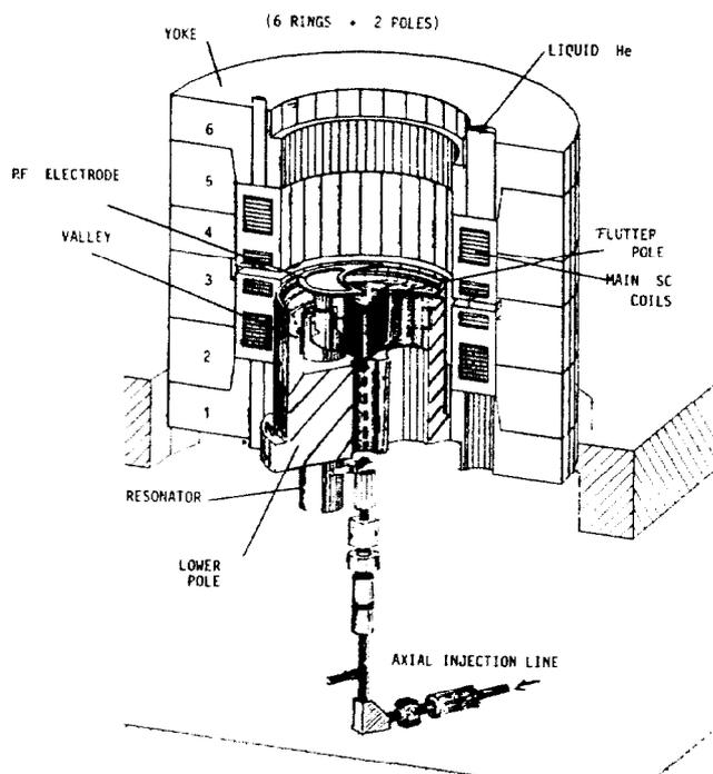
Fig.1 - Simplified cutaway view of the magnet assembly.
