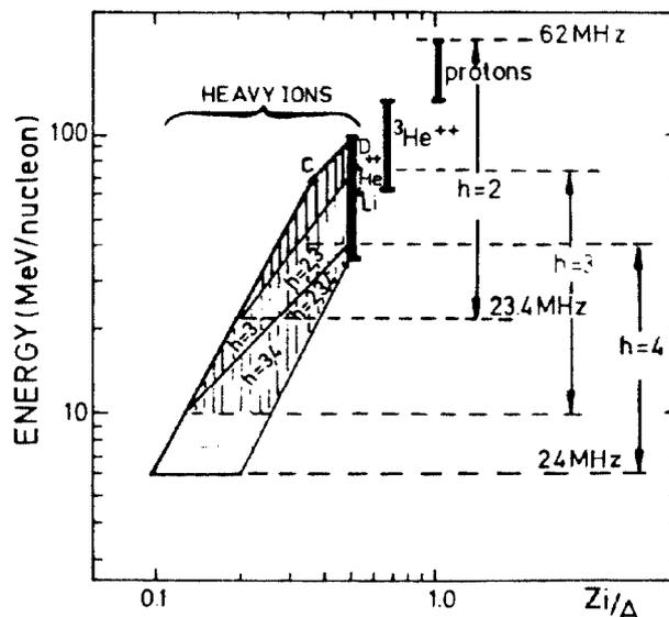
Fig.2 - Ions energy versus Z/A and boundaries the operating range of the RF frequency.
