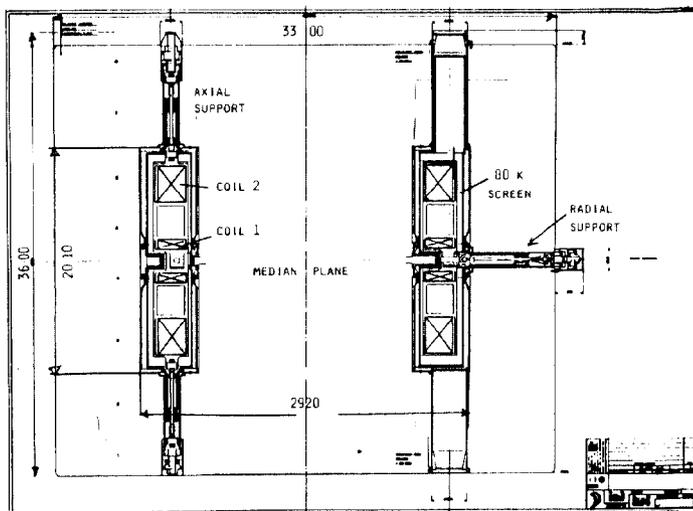
Fig.5 - Overall view of the cryostat and the coils. All dimensions are in mm.
