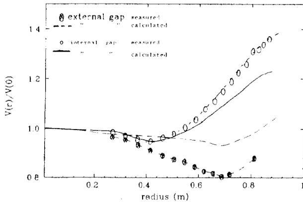
Fig.7 - Comparison between calculated and measured voltage distribution at 62 MHz.
