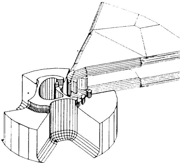
Fig. 8 - View of the central region of the cyclotron AGOR.
