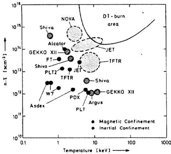
FIG.1. Lawson diagram showing the product of density  $n$  and confinement time  $\tau$  versus the temperature achieved in some magnetic and inertial fusion devices.
