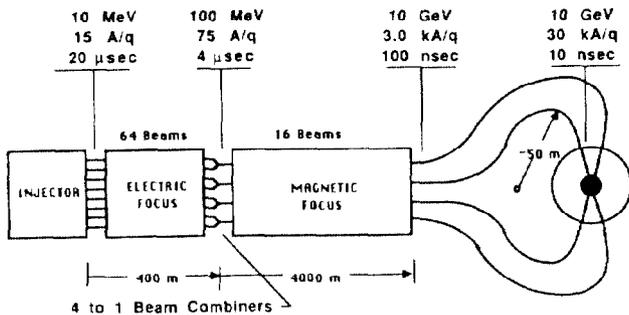
Figure 2: INDUCTION LINAC DRIVER (A=200, q=3)
